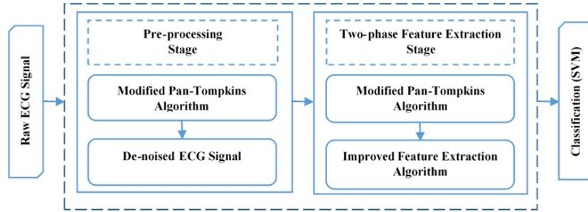
**Figure 2:** Block diagram of the two-stage feature extraction approach.
