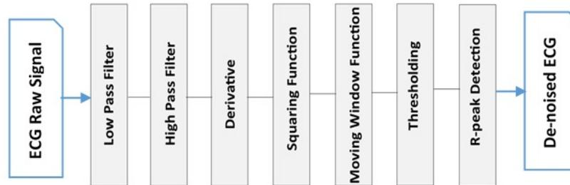
**Figure 1:** Modified Pan-Tompkins Algorithm Process.
